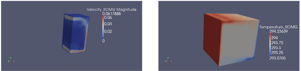
Fig. 5. ROM-G-Learning solution profile (left-side: velocity, right-side: temperature) – Case one.
