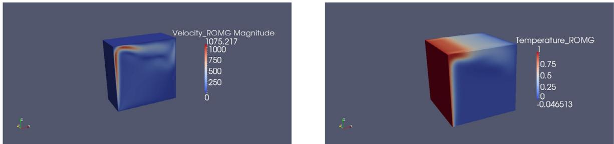
Fig. 10. ROM-G-Learning solution profile (left-side: velocity, right-side: temperature) – Case two.
